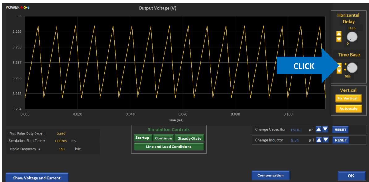
Fig. 2.7: POWER 4-5-6 Expanded Output Voltage Waveform
