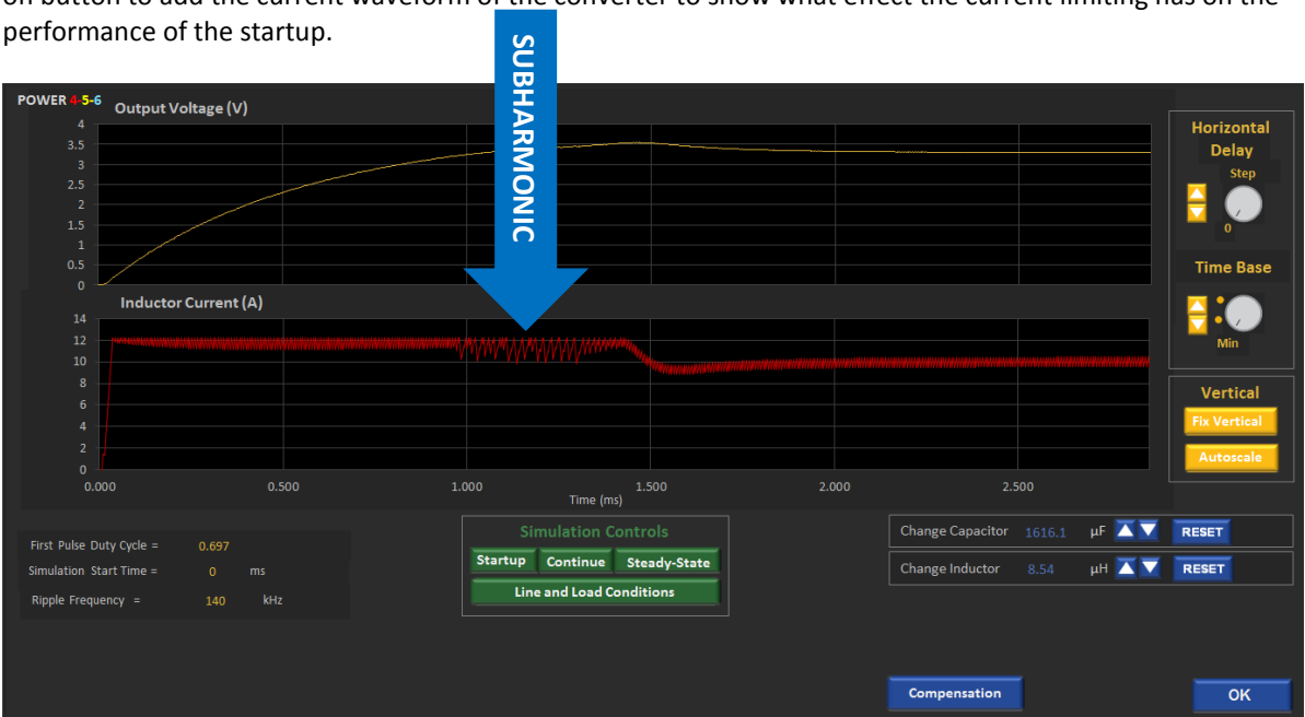
Fig. 2.9: POWER 4-5-6 Start Up Simulation Voltage and Current Waveforms
