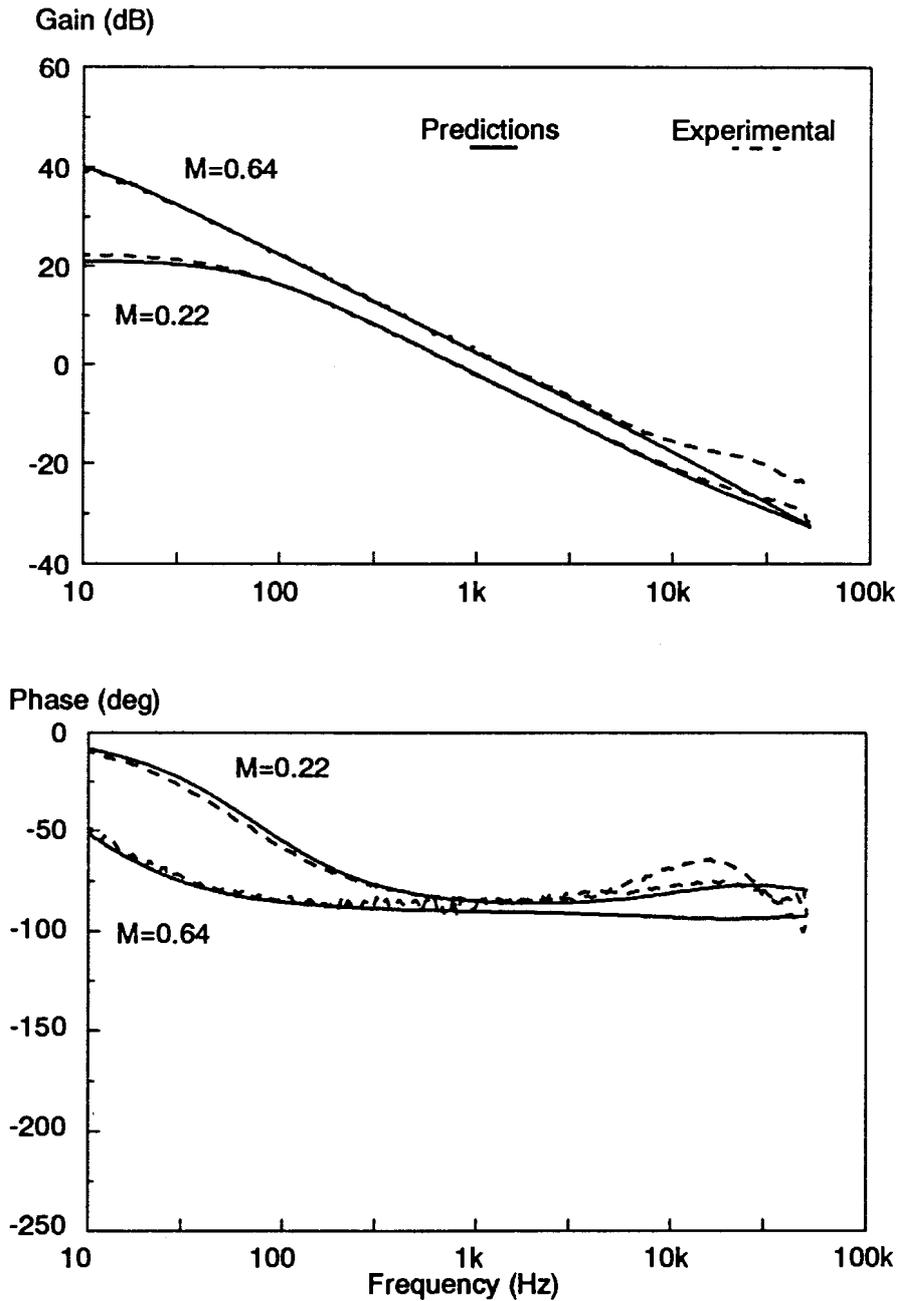
**Figure 5.25.** *Control-to-Output Transfer Function for Buck Converter (DCM): As the conversion ratio of the converter increases, the dominant pole of the system moves towards the zero axis. When the conversion ratio exceeds 0.67, this pole crosses into the right-half plane, and the system becomes unstable.*
