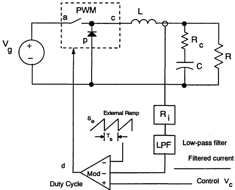
**Figure 2.7 "Average" Current-Mode Control:** The sensed inductor current, or switch current, is processed by a low-pass filter. If the filtering is sufficient, average models work well for this scheme. This is not analyzed in this dissertation.
