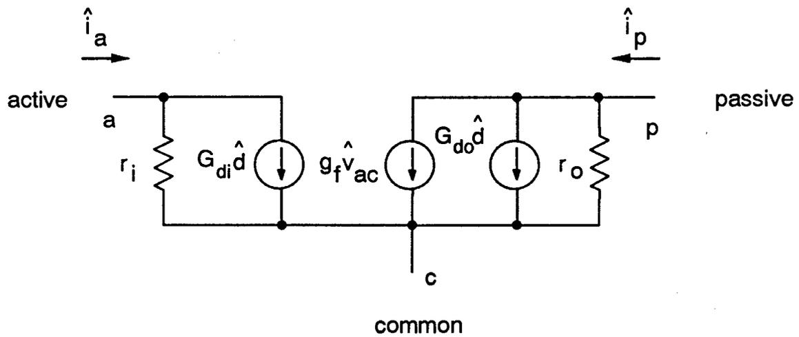
**Figure 4.10.** *PWM Switch Model for Discontinuous-Conduction Mode.: The PWM switch model for DCM is different from the model for CCM. It is invariant for all PWM converters.*
