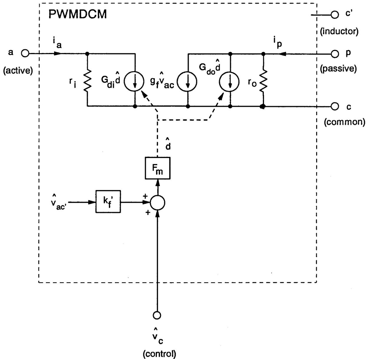
**Figure B.2.** *Small-Signal Controller Model for Voltage-Mode and Current-Mode Control in DCM: The controller model, referred to as PWMDCM, incorporates the feedback control and power stage PWM switch model for discontinuous conduction mode into one convenient subcircuit.*
