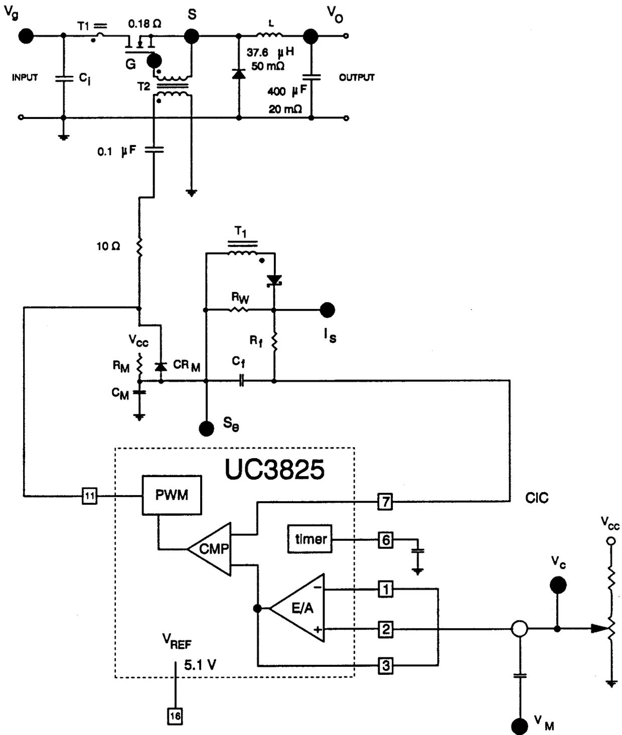
**Figure 5.2. Experimental Buck Converter for Small-Signal Measurements:** An experimental circuit was built to confirm the predictions of the model with measured data. The essential components and functions of the current-mode control are shown in this circuit diagram.
