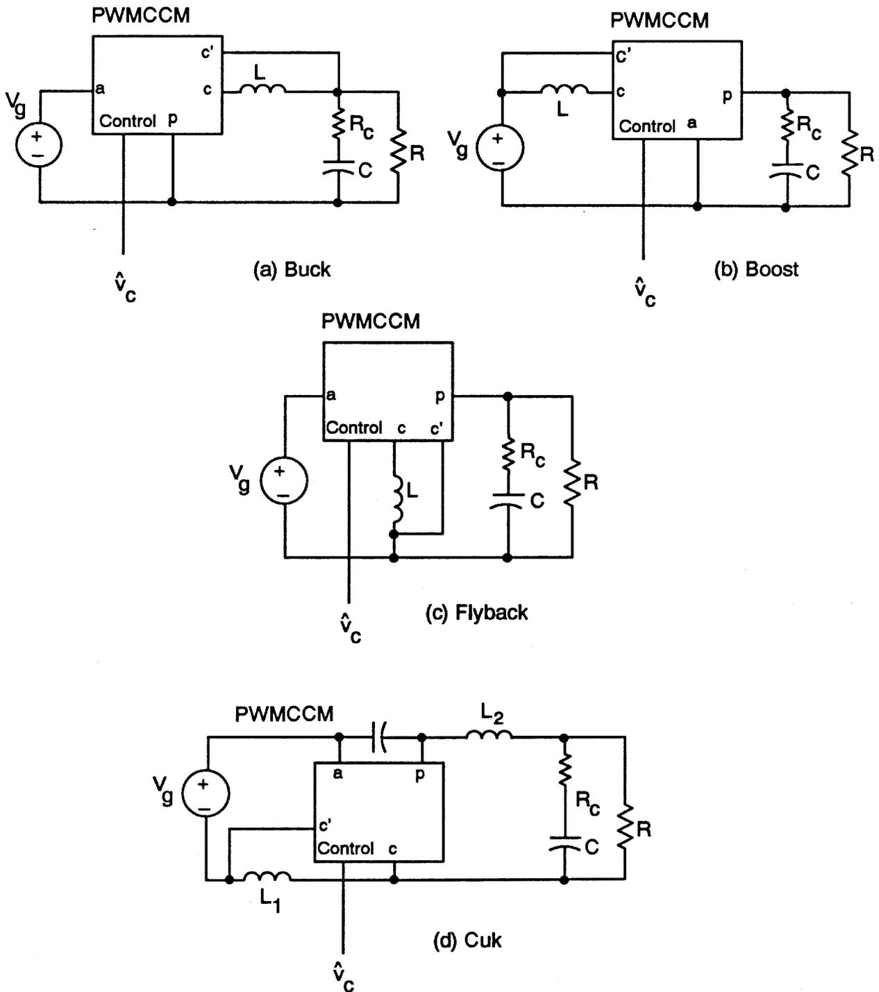
**Figure B.3.** *Small-Signal Controller Placed in Different Converters: Connections of the controller of Fig. B.1 in four types of PWM circuits are shown. Care must be taken with polarities of current sensing for the boost converter, and with the correct value of equivalent inductance for the Cuk converter.*
