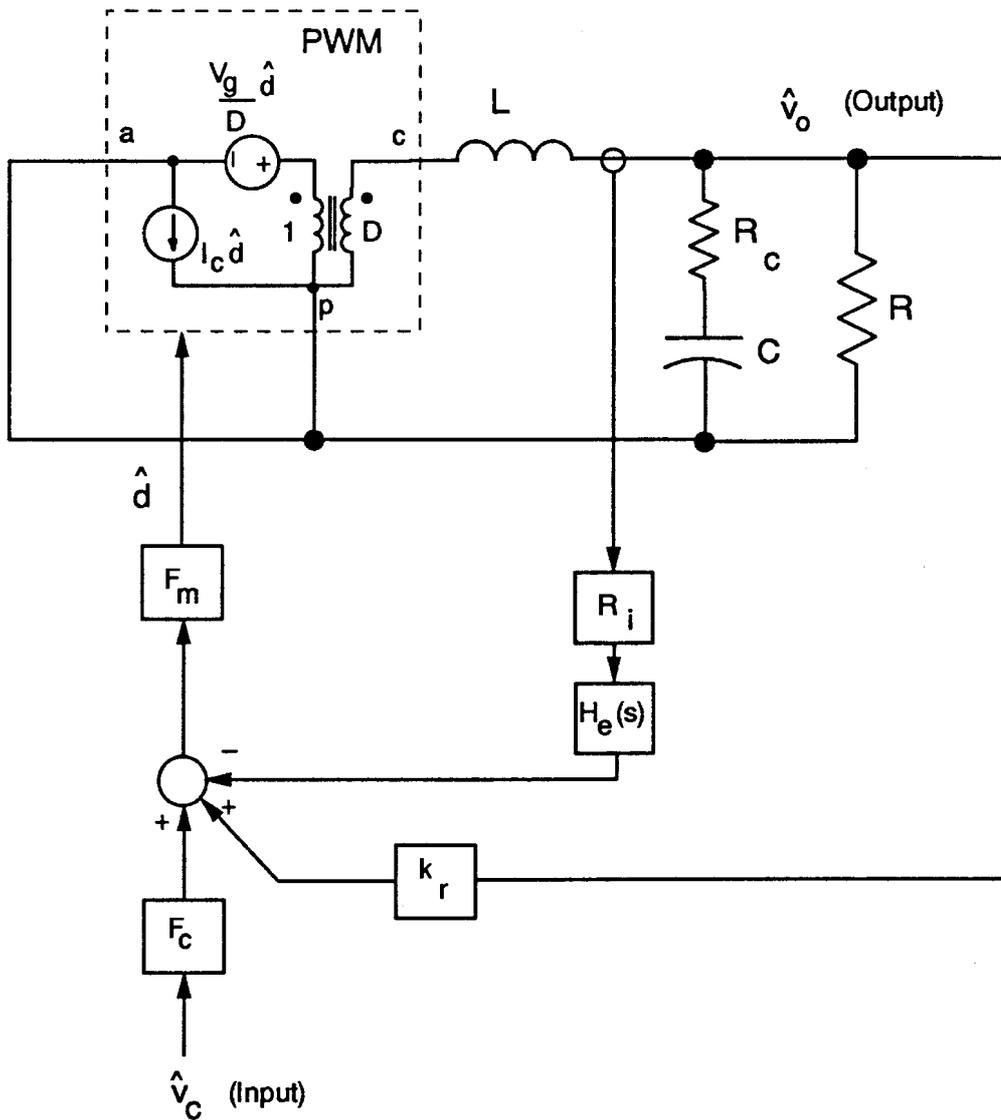
**Figure 5.6. Buck Converter with Current-Loop Closed:** The closed current loop of the system changes the control-to-output characteristics. Most designers prefer to use the control-to-output transfer function to select the closed-loop compensation.
