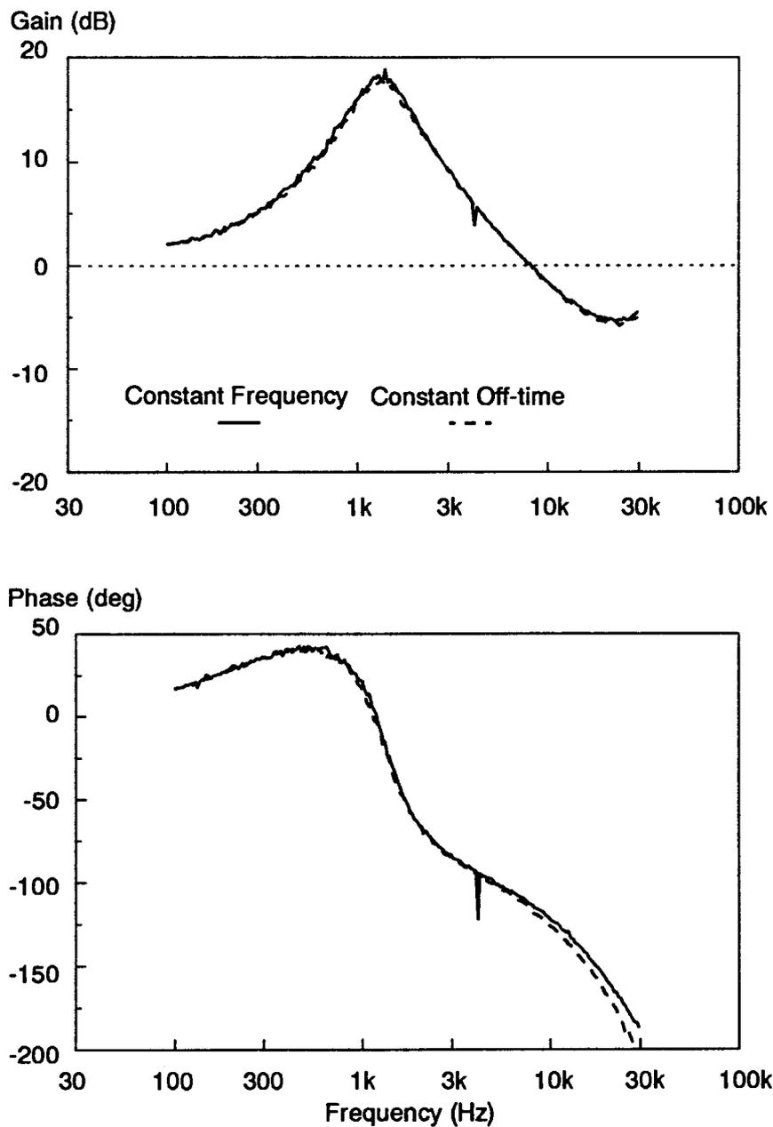
**Figure 5.19.** *Current Loop-Gain Measurement for Constant Off-Time:* The current loop gain for the constant off-time system is identical to the current-loop gain with constant-frequency control with an external ramp equal to the off-slope of the current signal. This loop gain remains invariant with duty cycle for the constant off-time control, remaining stable under all conditions.
