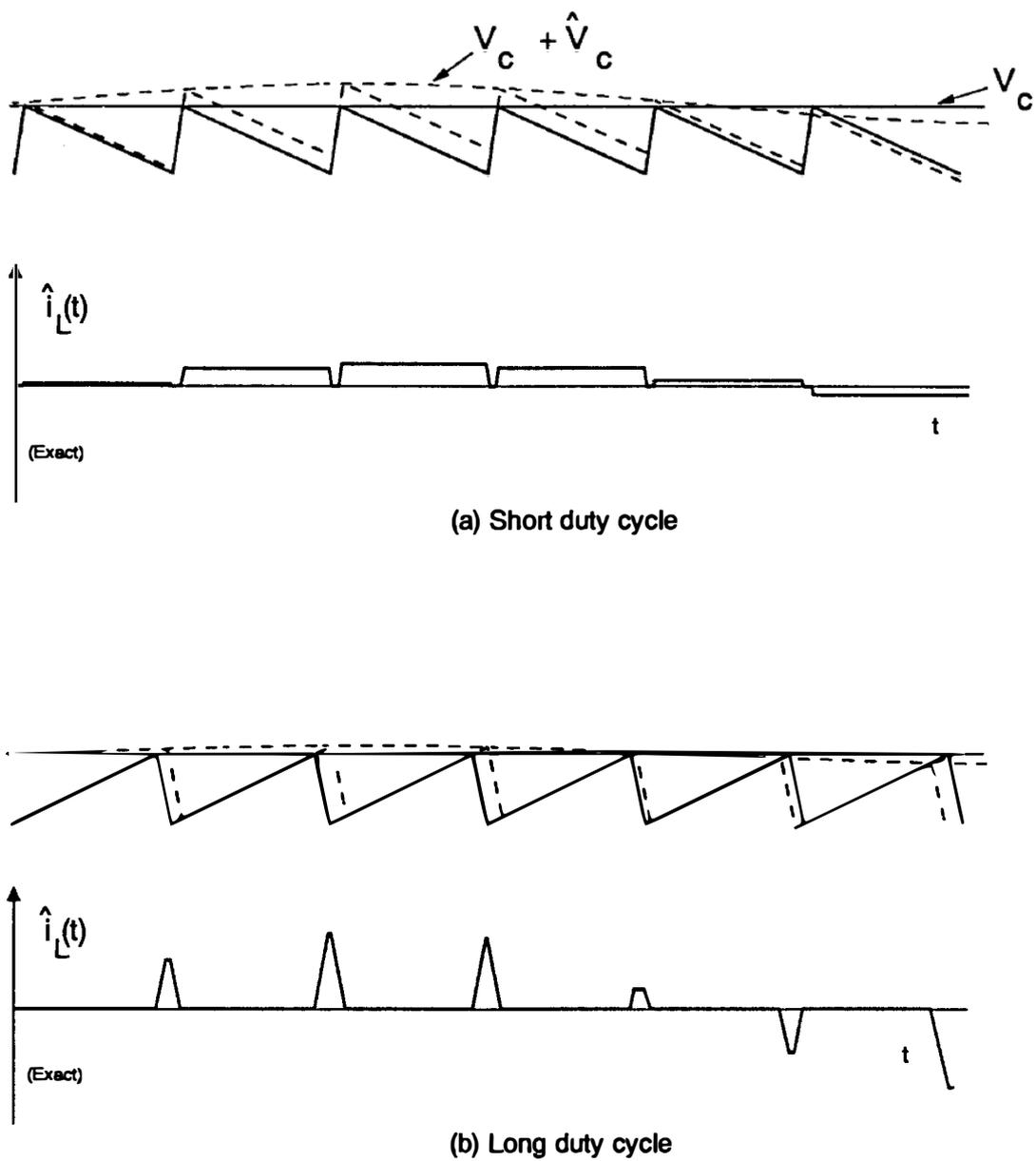
**Figure 3.13. Constant Off-Time Responses at Different Duty Cycles:** At duty cycles
