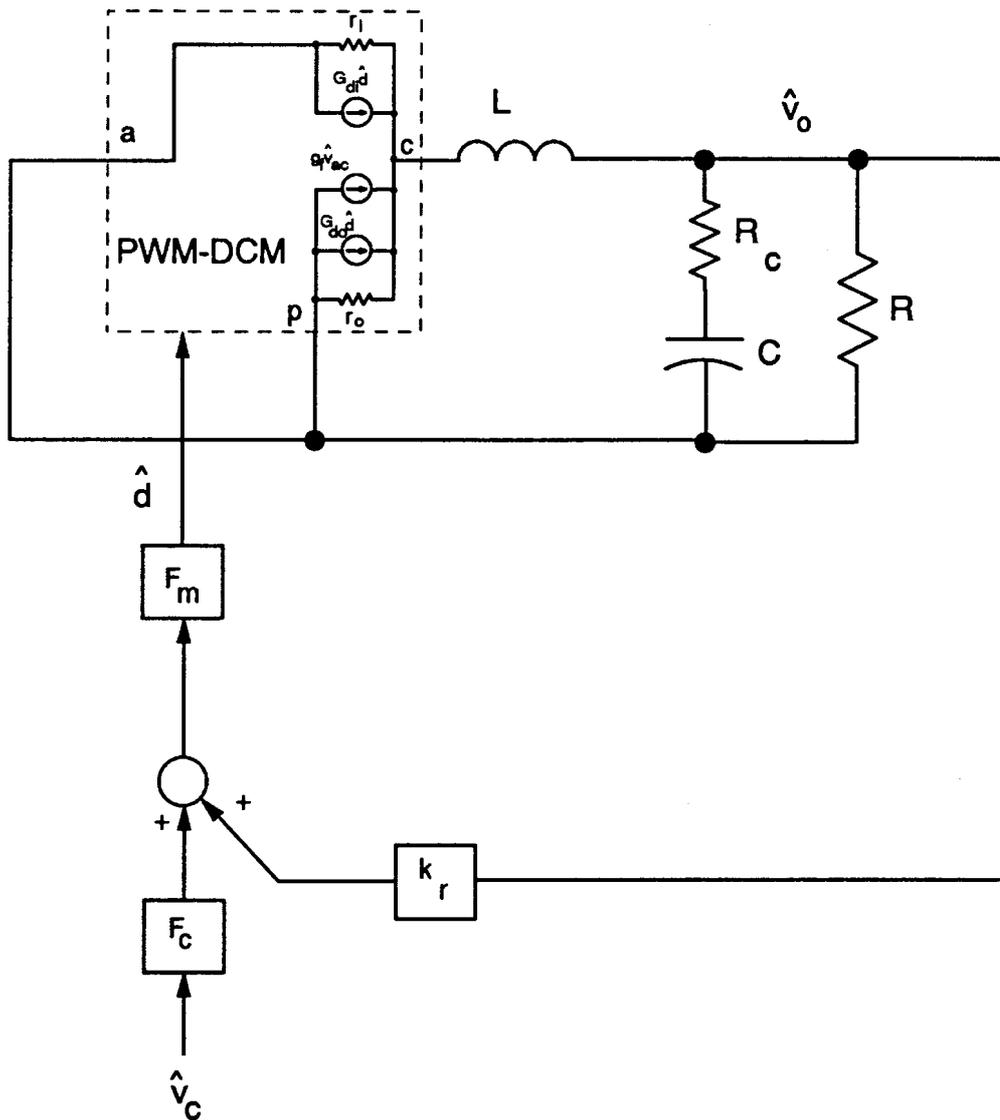
**Figure 5.24.** *Circuit for Control-to-Output Derivation for the Buck Converter in DCM: The power stage operating in DCM is replaced with the PWM switch model of Fig. 4.10, and the feedforward gain  $k_r$  is given in Table 4.7. Feedforward gain  $k_f$  does not appear since input perturbations are zero. Feedback of the inductor current does not explicitly appear in the small-signal model.*
