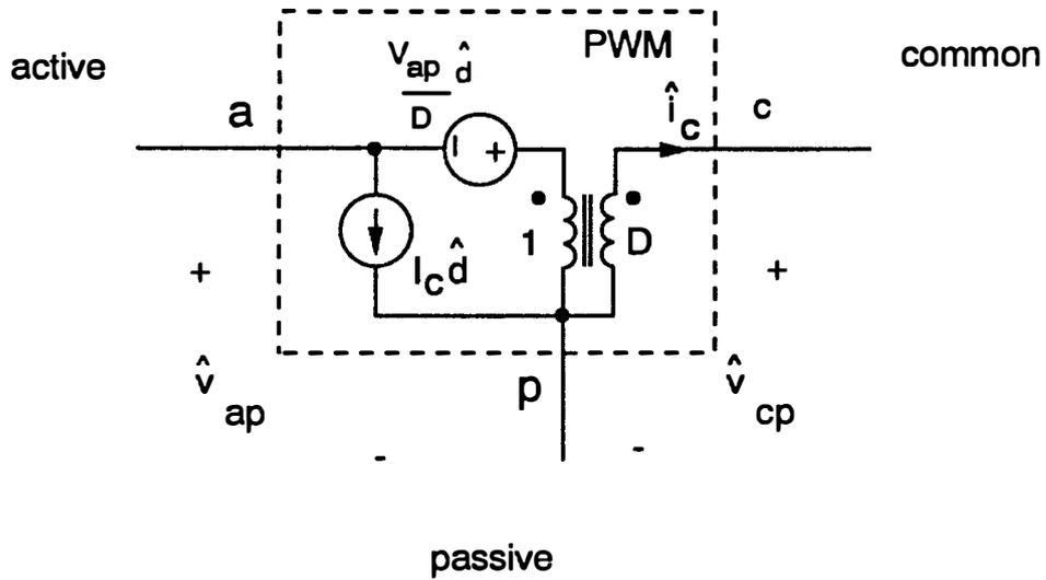
**Figure 2.9. PWM Switch Model for Continuous-Conduction Mode:** This invariant model replaces the nonlinear switching block in the PWM converters to provide a simple, convenient small-signal model.
