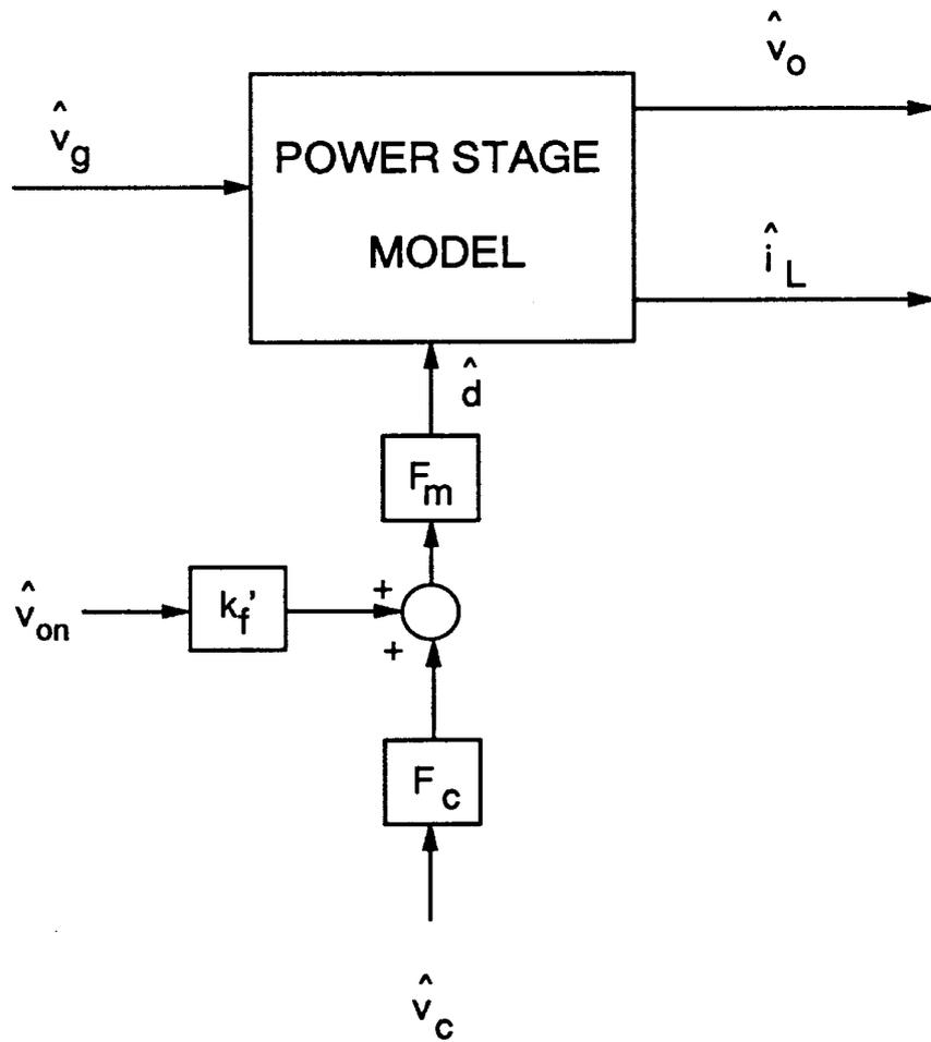
**Figure 4.13.** *Invariant Model for Current-Mode Control (DCM): Only the feedforward gain,  $k_f'$ , from the on-time voltage is needed in this form of the model. The value of this parameter is the same for all converters being modeled.*
