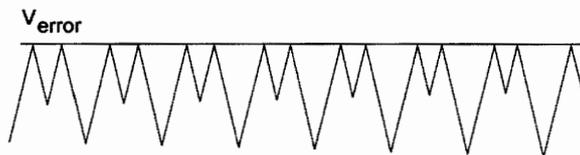
Fig. 3: Subharmonic oscillation waveforms.
