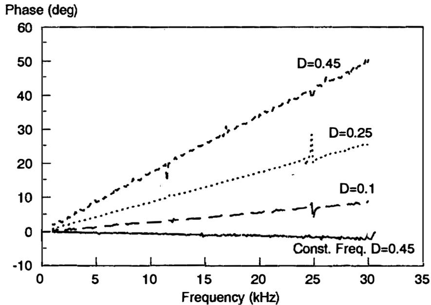
**Figure 3.10. Constant Off-Time Modulator Phase Measurement:**
