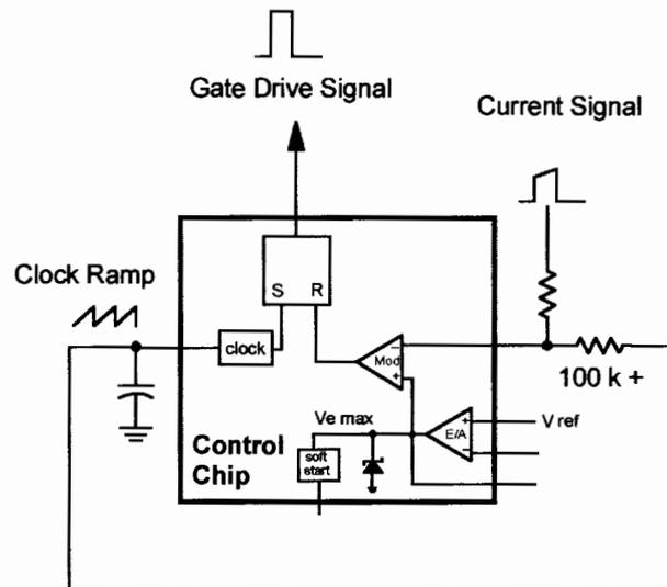
Figure 10: Resistive summing of the timing ramp and current signal for ramp addition. This circuit is NOT recommended. The clock signal is very sensitive to loading and noise, and can lead to power supply failure if it is corrupted.
