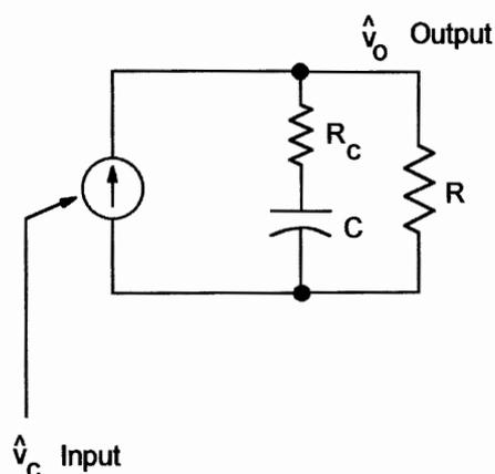
Fig. 2: Simplest small-signal model – current source feeding the load.
