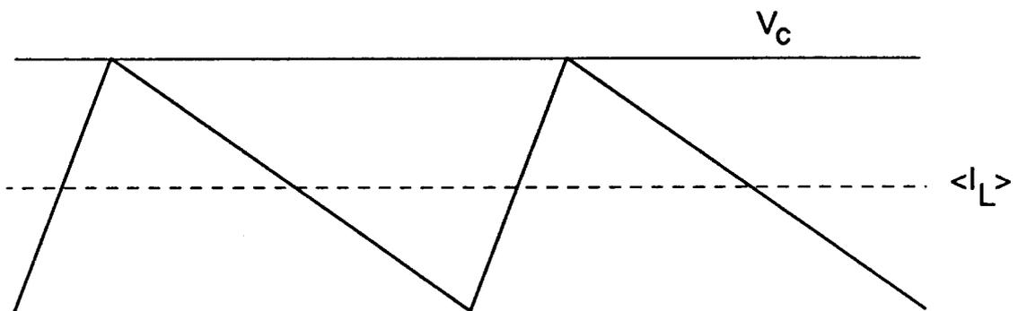
**Figure 5.14.** *Steady-State Waveforms of the Buck Converter with No External Ramp:* As the input line is increased, the steady-state ripple current is also increased. Since the peak of the current is regulated, the average value of the current, and hence the output voltage, is decreased.
