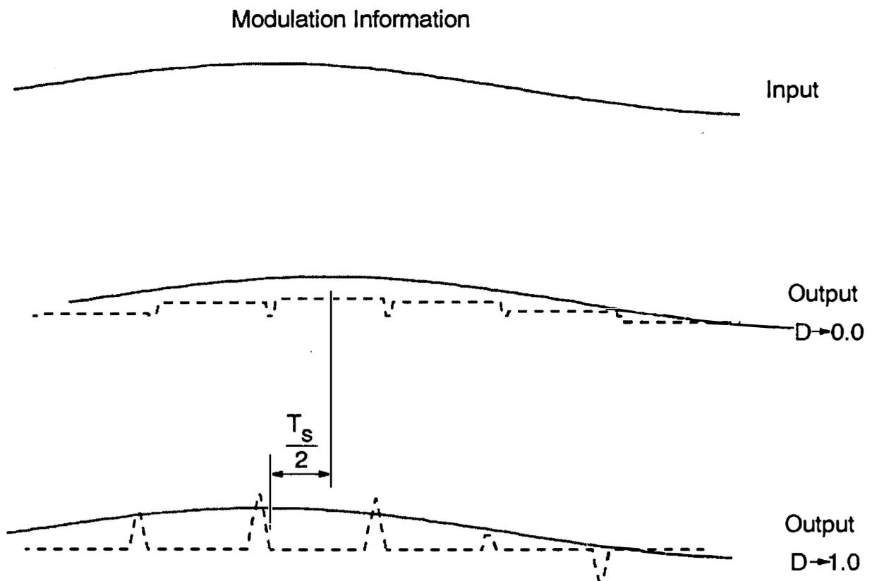
**Figure 3.14. Modulation Information Carried by Constant Off-Time Modulator:**
