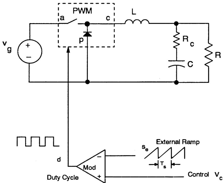
**Figure 2.1. Buck Converter with Voltage-Mode Control:** The duty cycle control signal is provided by a sawtooth ramp intersecting a control voltage threshold. The model for this control system is well represented by existing average techniques, provided that the control signal is continuous.
