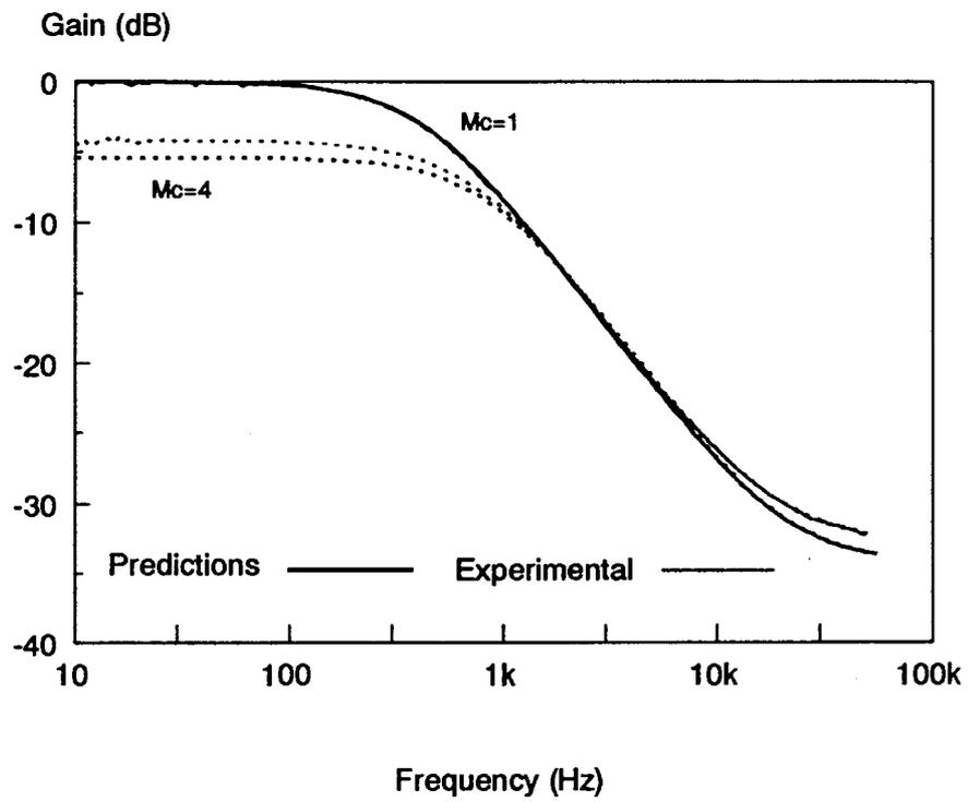
**Figure 5.18. Output Impedance of the Buck Converter - Experimental Results: Experimental and predicted measurements agree well.**
