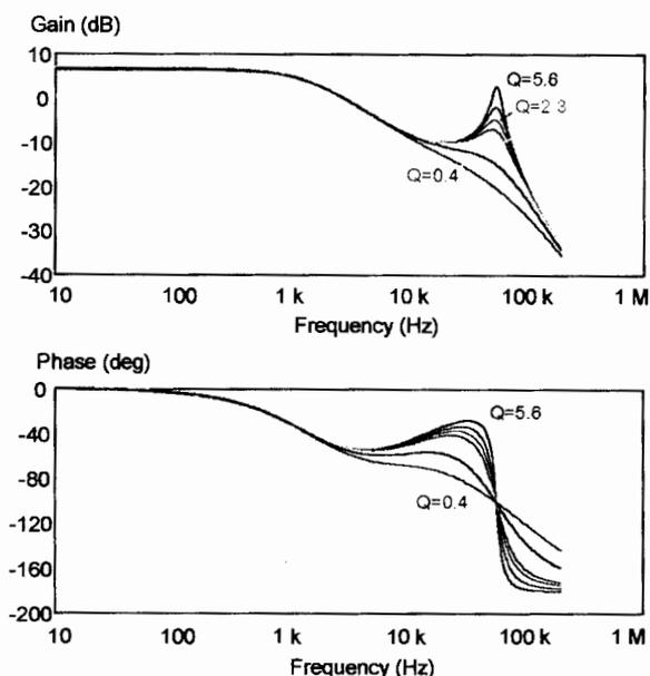
Fig. 5: Power stage transfer functions plotted up to the switching frequency. Notice the obvious double-pole characteristic centered at half the switching frequency.
