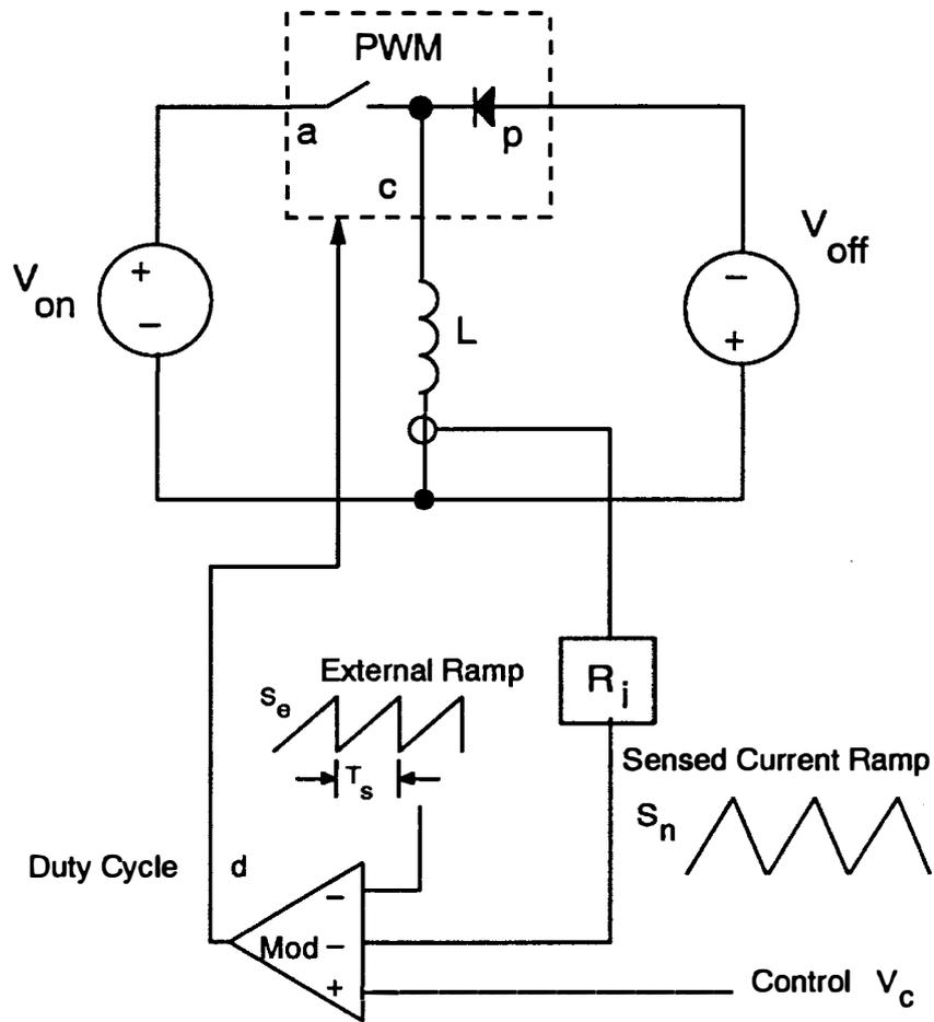
**Figure 3.3. Generic Current-Mode Cell:** The generic cell represents all of the converters with current-mode feedback. The input and output voltages are now the quantities  $V_{on}$  and  $V_{off}$ , which are combinations of the input and output voltages of the different PWM converters.
