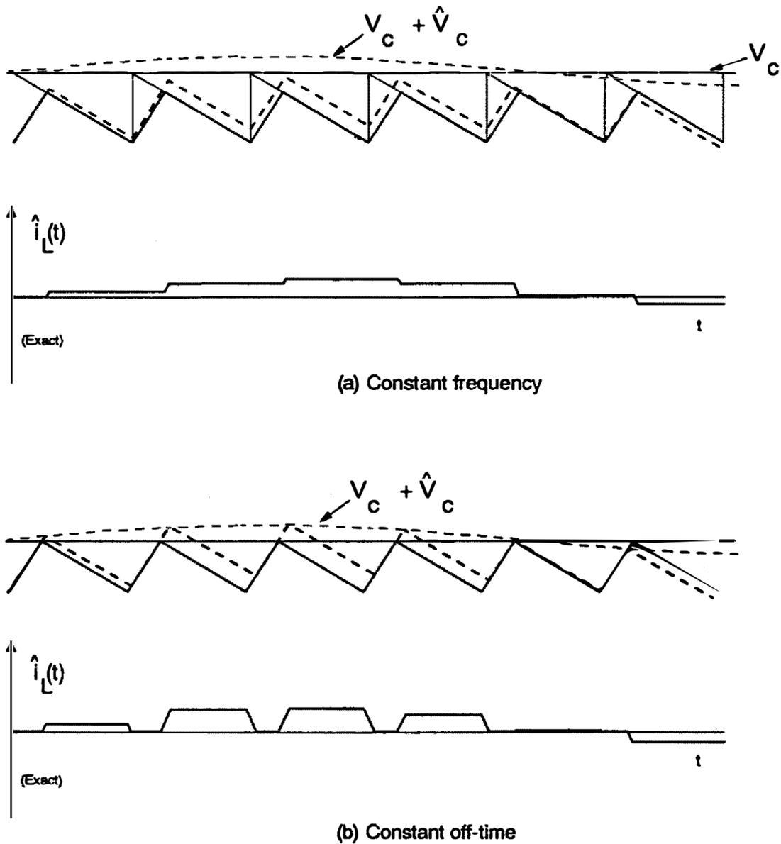
**Figure 3.12. Comparison of Constant-Frequency and Constant Off-Time Control:**
