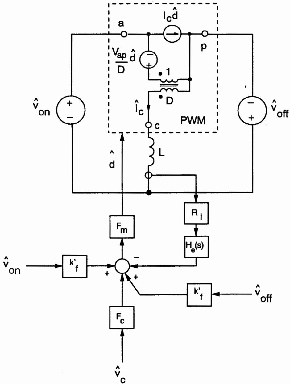
**Figure 4.7. Small-Signal Model for the Generic Current Cell:** The input and output voltages of the generic cell are  $v_{on}$  and  $v_{off}$ , respectively. For the flyback converter, these are equal to the input and output voltages, and in general are linear combinations of the input and output voltages.
