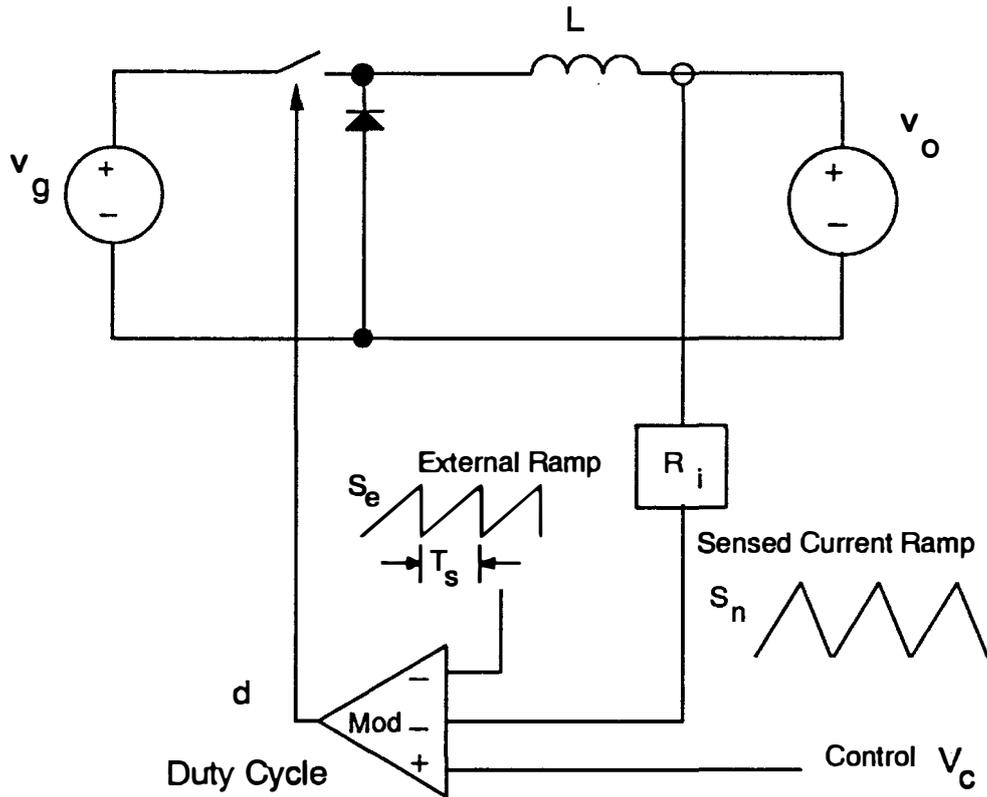
**Figure 2.14. Sampled-Data Modeling Approach:** A simple buck converter was modeled at high frequencies using sampled-data techniques. This was able to explain some of the phenomena of current-mode control, but the complexity of the modeling led researchers to abandon this technique.
