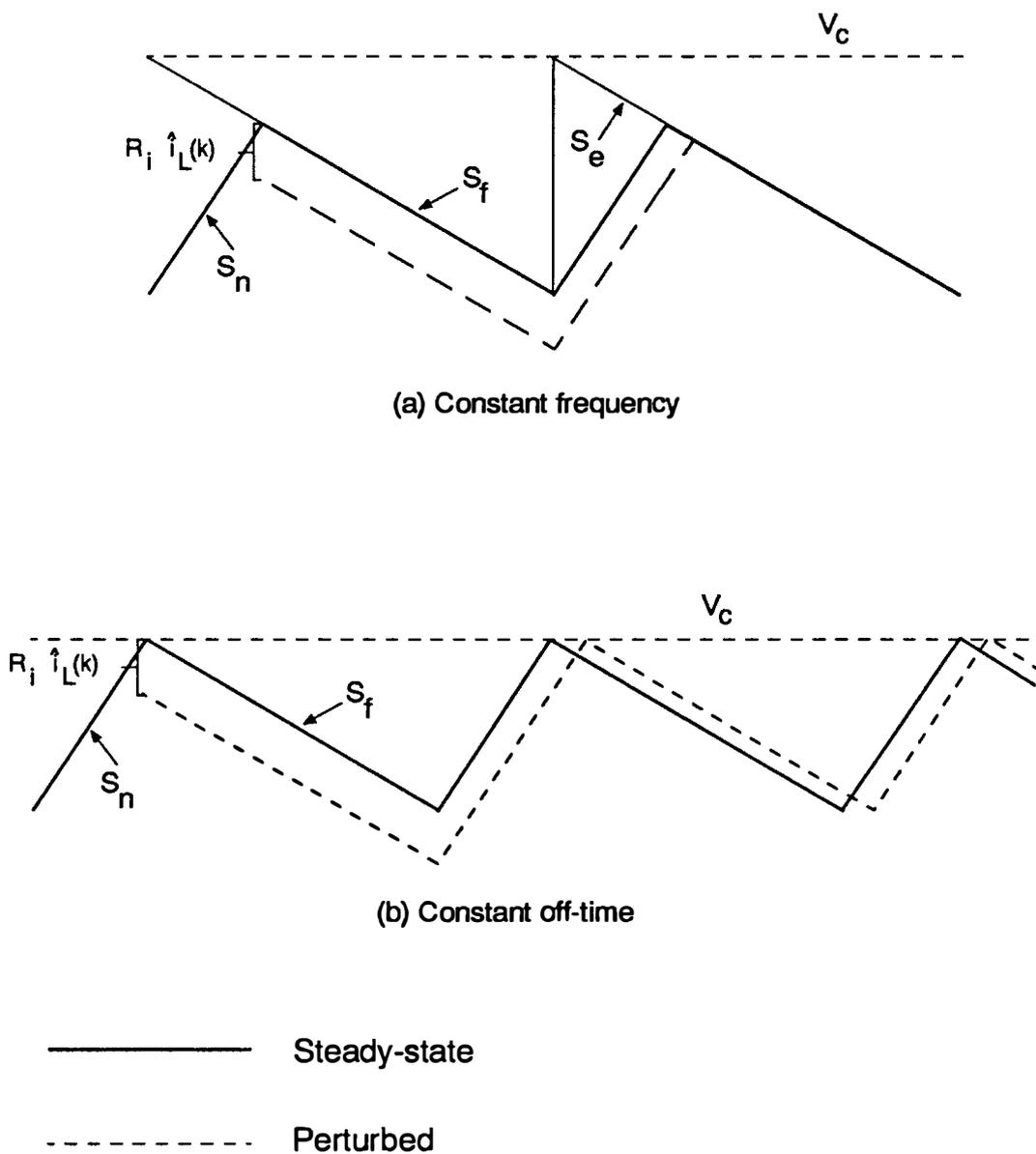
**Figure 3.11. Comparison of Constant-Frequency and Constant Off-Time Control:**
