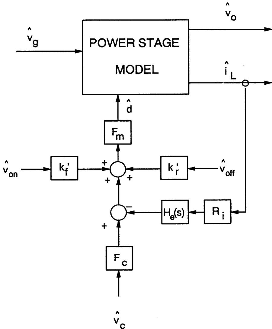
**Figure A.1. Small-Signal Model for Continuous-Conduction Mode:** The model shown in this figure is invariant for all PWM converters, and can be used for current-mode or voltage-mode control ( $R_i = 0$ ). All transfer functions, including the current-loop gain, can be generated with this model. Parameter values for the model are given in Table A.1 for the different modulation strategies.
