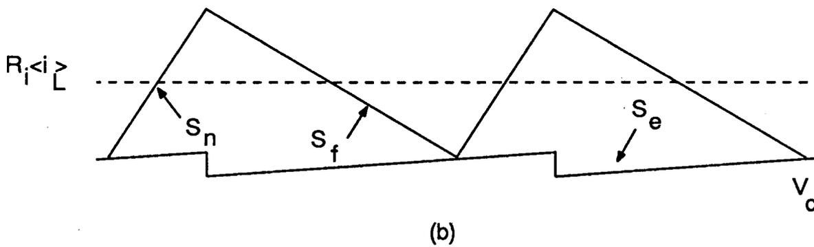
**Figure 4.4. Steady-State Modulator Waveforms:** The average inductor current,  $\langle i_L \rangle$  is related to the peak current and the ripple current. The ripple current is determined by the voltages across the inductor during the on and off times, and by the duty cycle.
