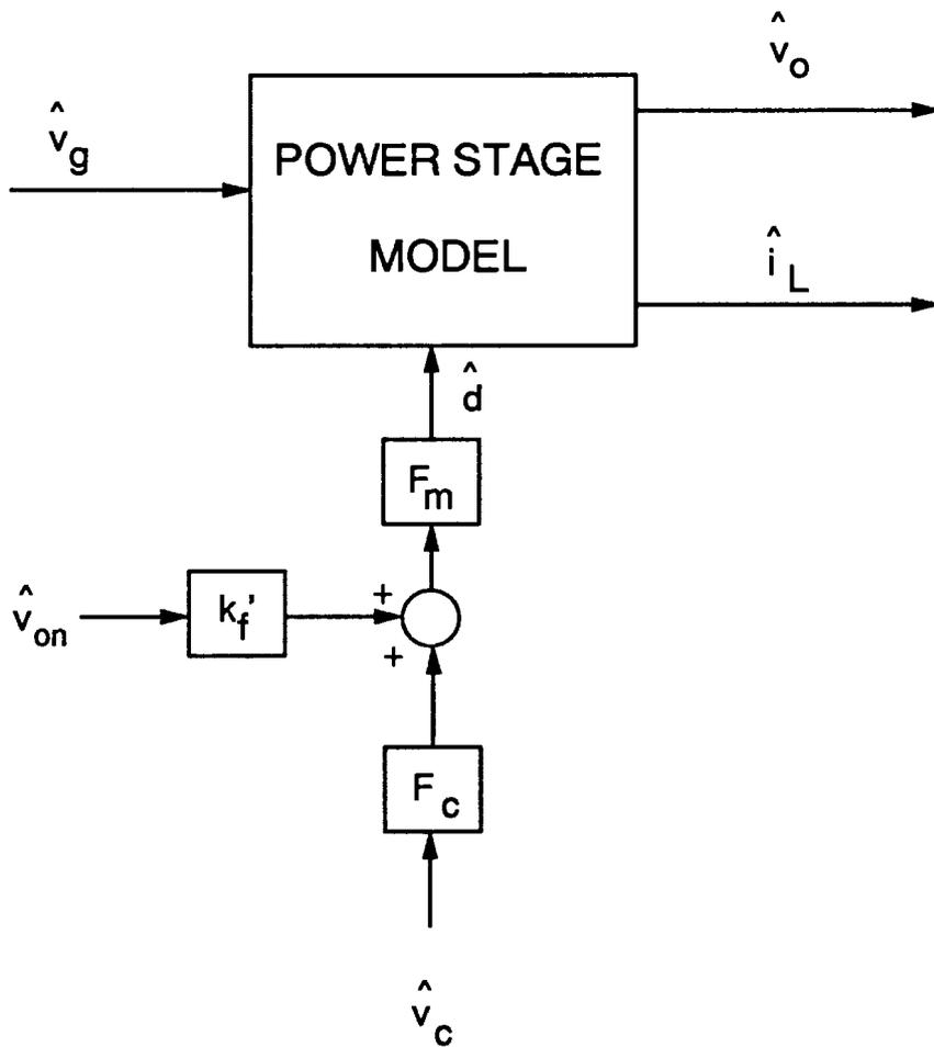
**Figure A.2. Small-Signal Model for Discontinuous-Conduction Mode:** This invariant model is used for all converters in DCM. It is valid for both current-mode and voltage-mode control. Notice that the current feedback does not explicitly appear in the model. Parameter values for the model are given in Table A.2.
