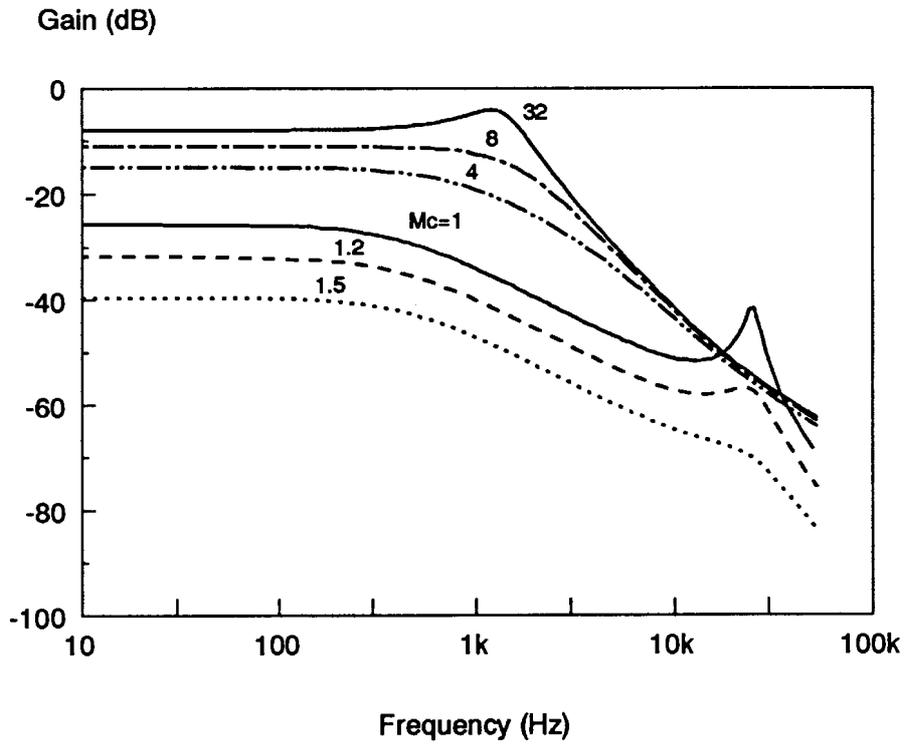
**Figure 5.13.** *Line-to-Output (Audio Susceptibility) of the Buck Converter: The audio susceptibility of the buck converter has the interesting feature of a null value for the critical value of external ramp. As the external ramp is increased through the null value, the phase of the audiosusceptibility changes sign.*
