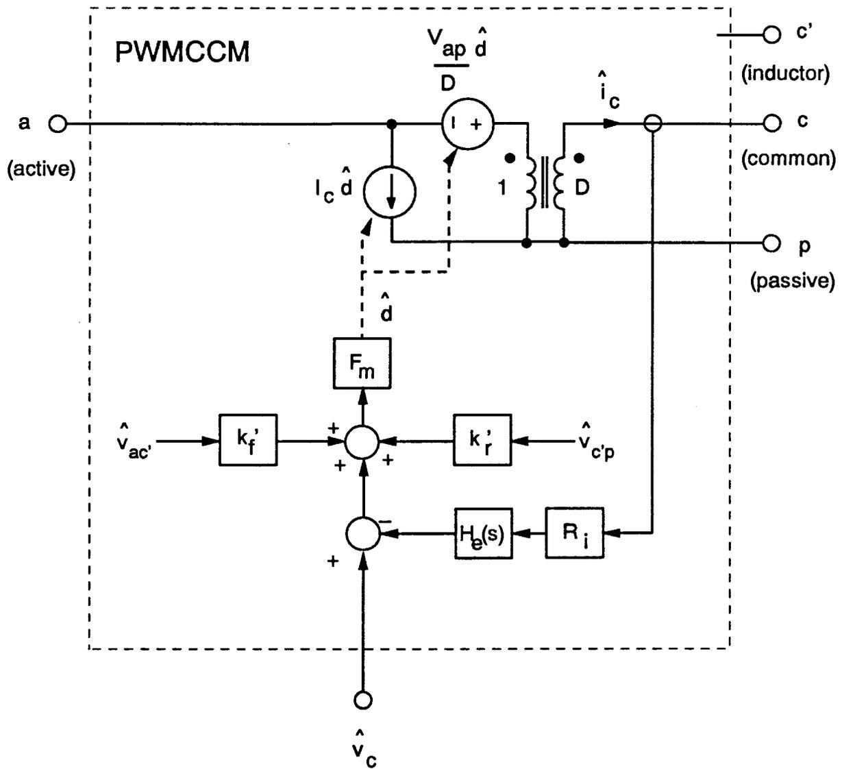
**Figure B.1. Small-Signal Controller Model for Voltage-Mode and Current-Mode Control in CCM:** The new controller model, referred to as PWMCCM, incorporates the feedback control and power stage PWM switch into one convenient subcircuit. Five connections must be defined for the subcircuit.
