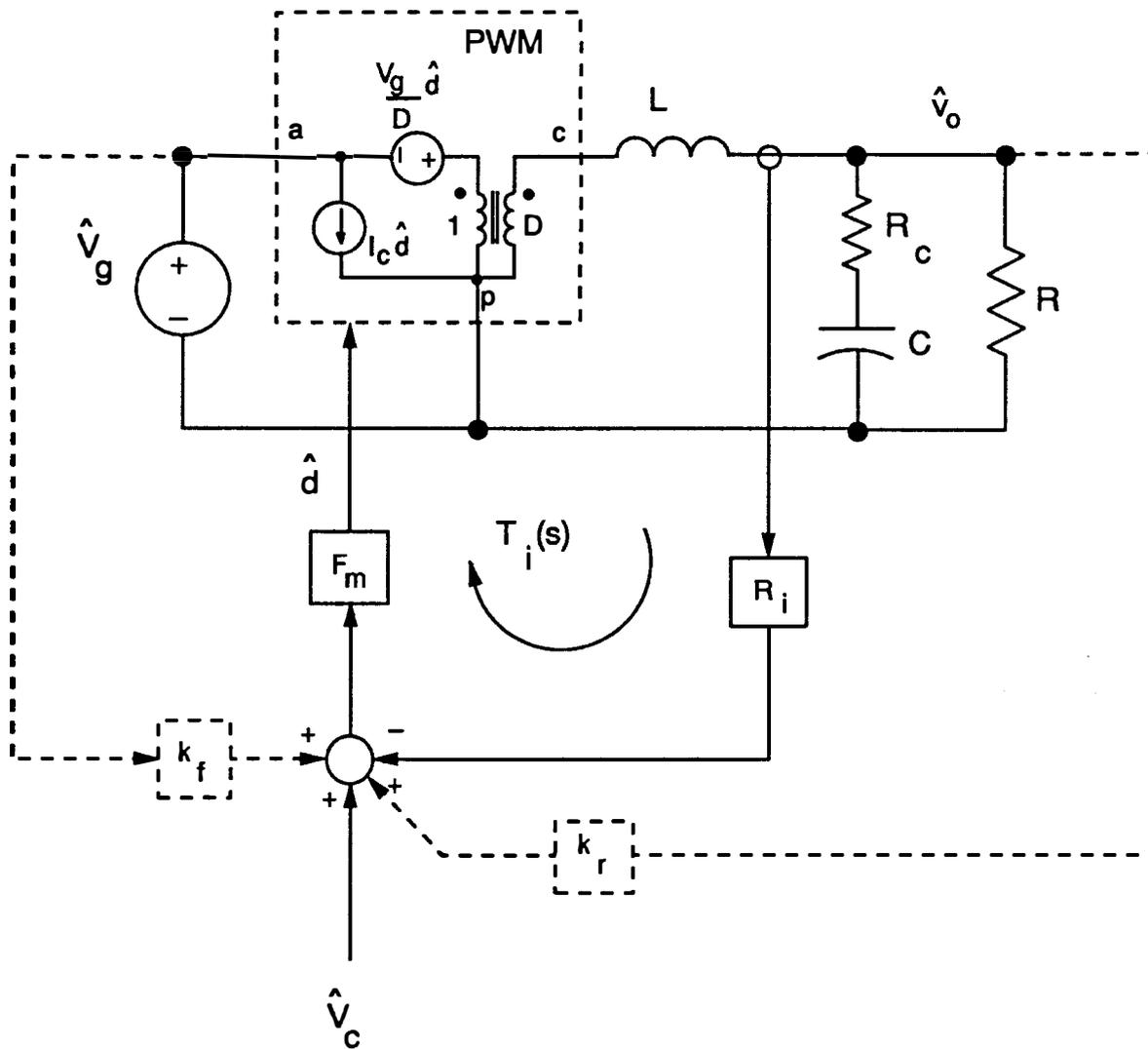
**Figure 2.12. Average Current-Mode Control Models:** The PWM switch is used to generate the power stage model. There are no frequency-dependent terms in the feedback of the inductor current. Some average models incorporate feedforward terms from input and output voltages.
