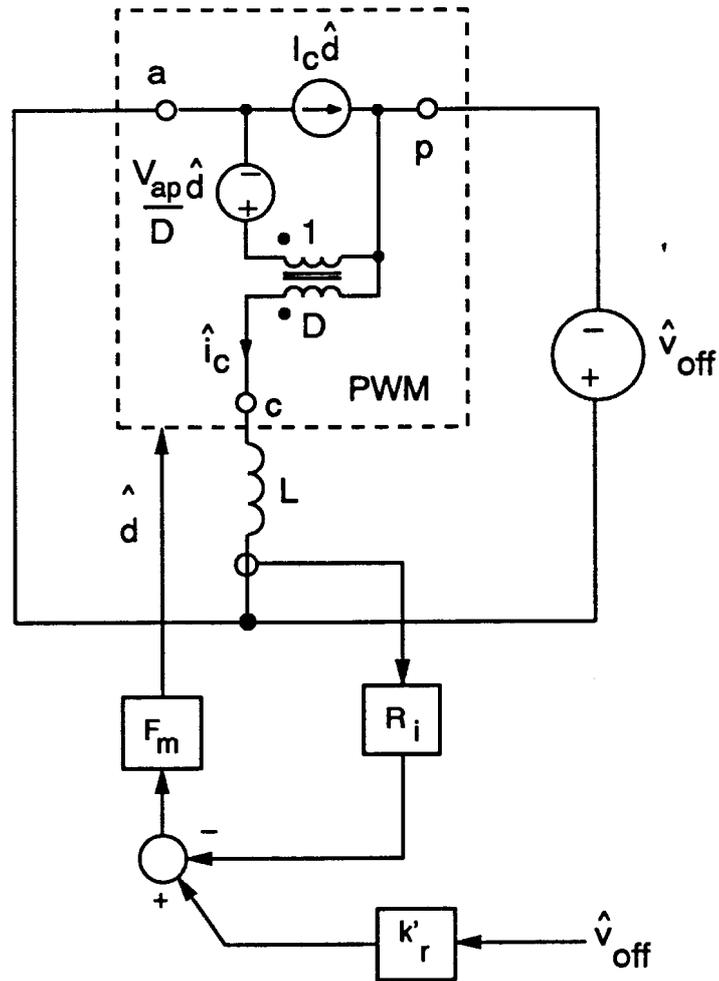
**Figure 4.9. Generic Current Cell with Fixed Voltage During On-Time:** The off-time voltage, again a linear combination of input and output voltages, is allowed to vary in this case, and the value of feedforward term,  $k'_r$ , is derived for all converters.
