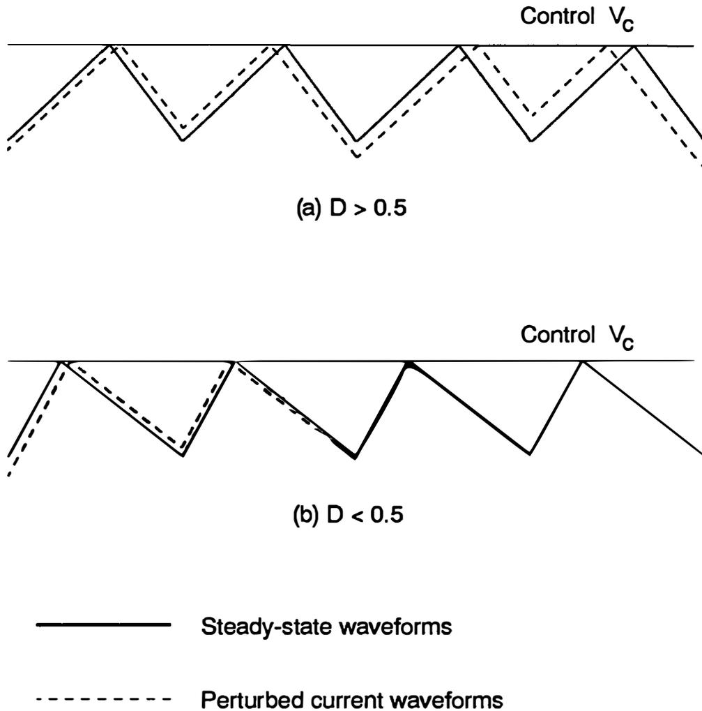
**Figure 2.11. Instability Observed with Constant-Frequency Controller:** With fixed-frequency control, and the clock initiating the on-time of the active switch, the closed current loop exhibits oscillatory behavior at half the switching frequency. This oscillation is damped at duty cycles below 0.5, and grows with larger duty cycles.
