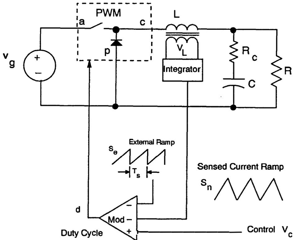
**Figure 2.3. Buck Converter with "SCM" form of Current-Mode Control:** A signal proportional to the inductor current is derived by integrating the voltage across the filter inductor. This approach provides a continuous current signal during on- and off-times of the switch, but dc information is lost.
