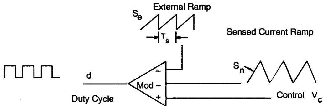
**Figure 2.5. Basic Structure of Current-Mode Controller:** Regardless of the current-sensing technique, both the CIC and SCM control achieve the same effect. The current signal is summed with an external ramp and compared with a control signal to provide the duty cycle to the power stage.
