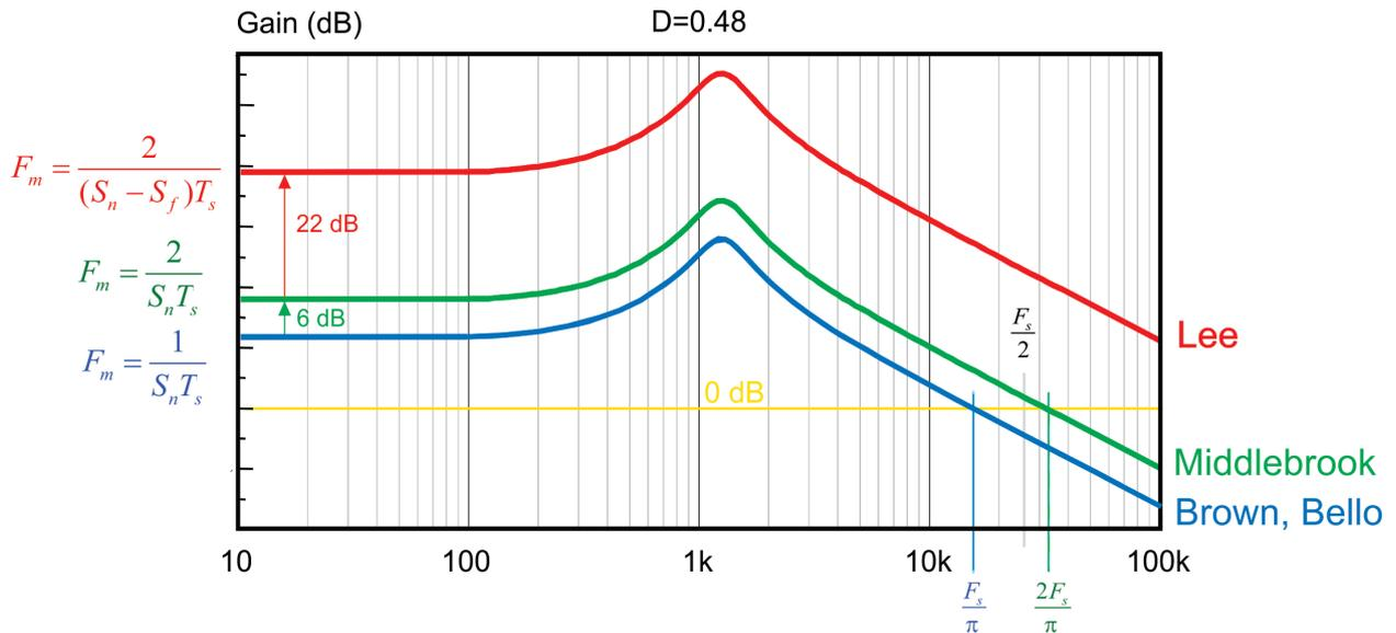
**Figure A3.1 Current-Mode Loop Gains from Lee, Middlebrook, and Bello (Brown):**
