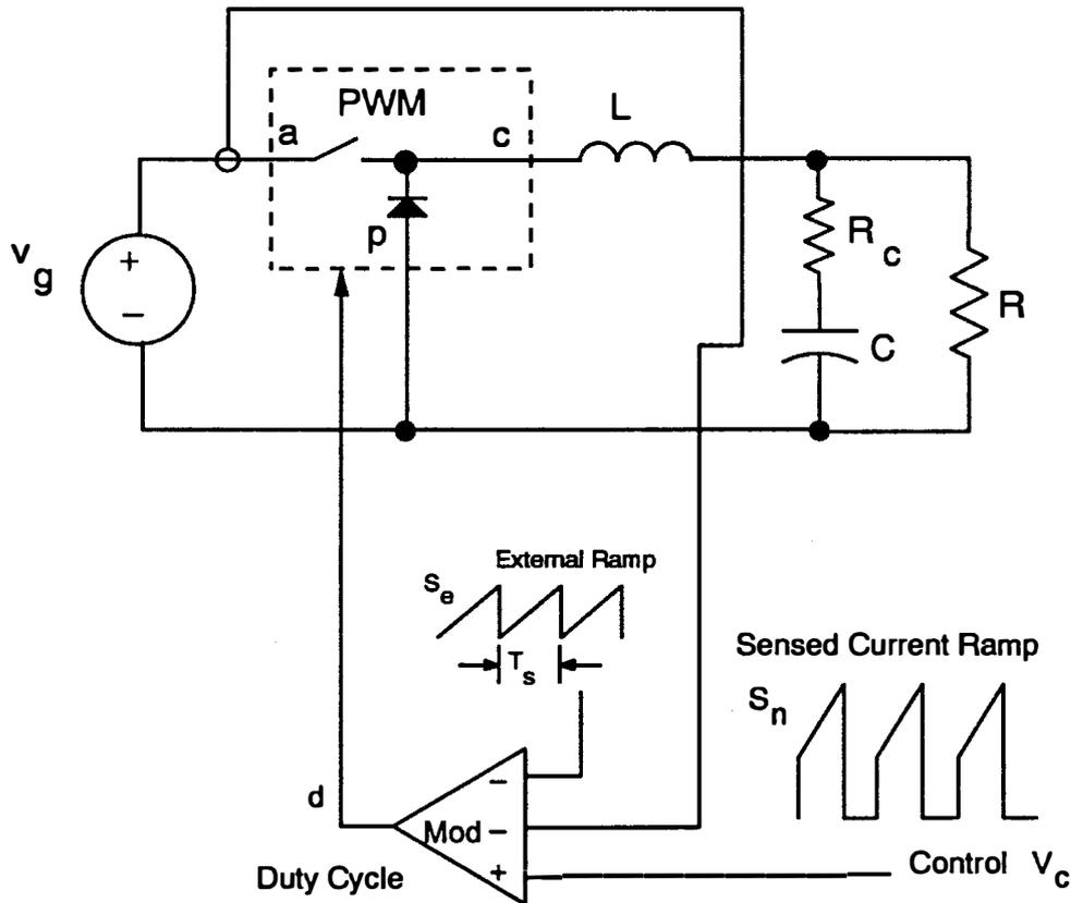
**Figure 2.4. Buck Converter with "CIC" form of Current-Mode Control:** In this scheme, the inductor current is sensed by a current transformer in series with the power switch. The current information is only available during the on-time of the switch. The de information of the current is preserved in this approach, providing inherent current limiting and current sharing of multiple modules.
