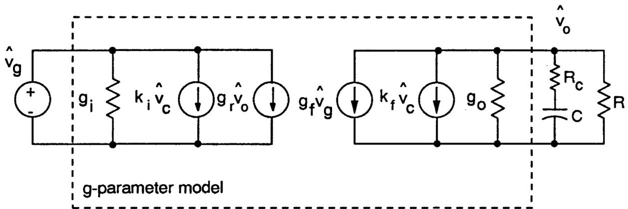
**Figure 2.13. Simplified Average Current-Mode Control Model:** Many previous modeling approaches assume that the current loop has sufficient gain and high enough crossover frequency to allow the low frequency model to be reduced to a single-pole model, without the inductor current.
