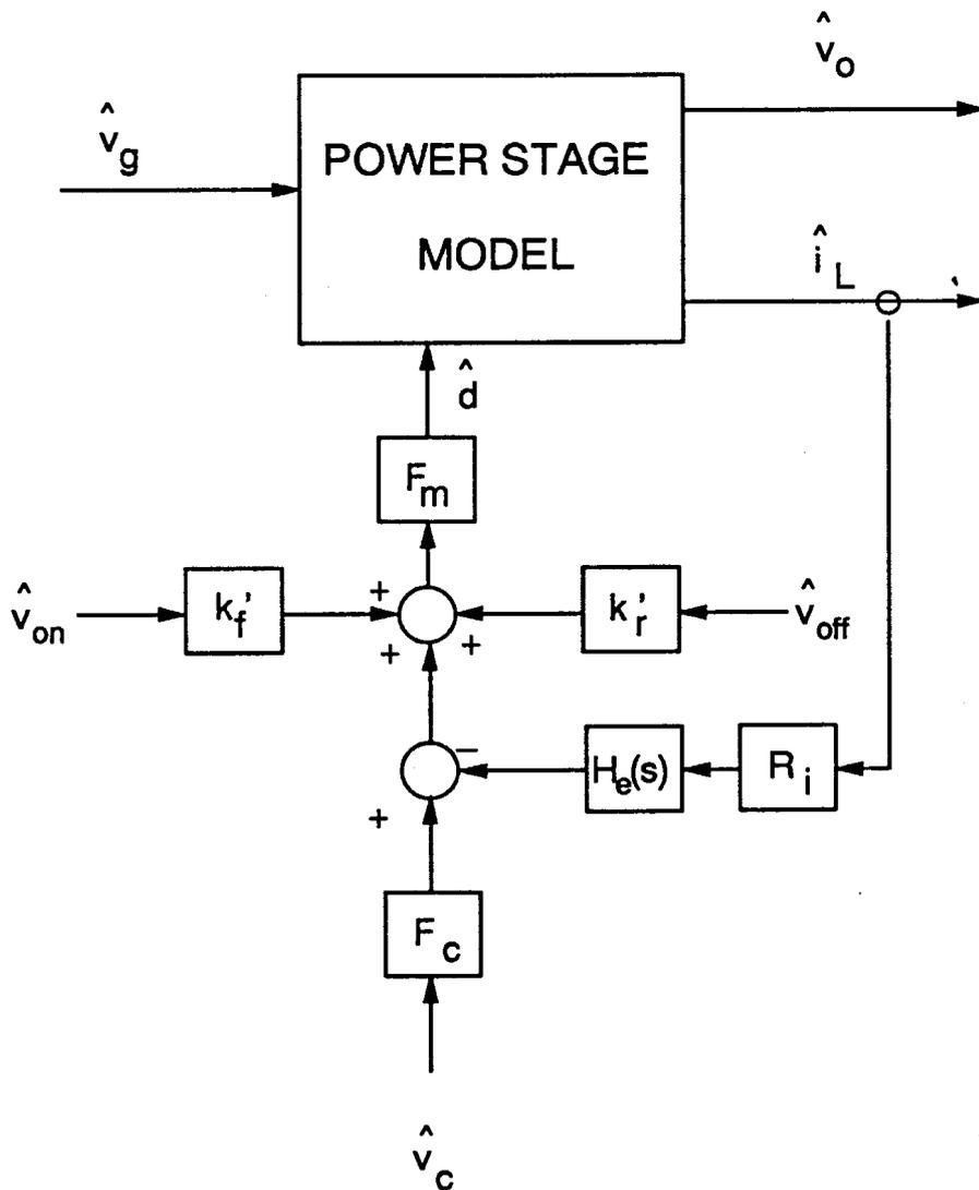
**Figure 4.6. Invariant Small-Signal Model for Current-Mode Control:** Feedforward terms in this model are from the on-time and off-time voltages of the current cell. This form of the model has the advantage of invariance. The values of  $k_f'$  and  $k_r'$  are constant, regardless of the power stage topology. This is more useful for circuit analysis programs.
