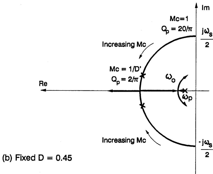
**Figure 5.8. Poles of the System with the Current-Loop Closed:** Unlike average current-mode models, the new current-mode model gives a control-to-output transfer function with three poles.
