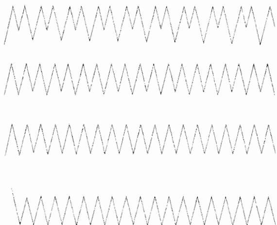
Fig. 6: Inductor current oscillation waveforms. Waveforms correspond to a  $Q$  of 7.6, 5.6, 2.3 and 0.7.
