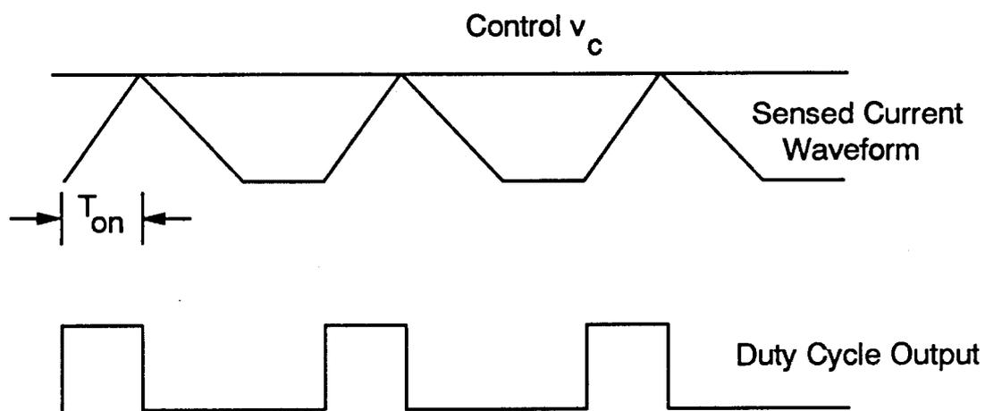
**Figure 4.11.** *Discontinuous-Conduction Modulator Waveforms for Current-Mode Control.:* The sensed current waveform added to an external ramp is compared with a control signal,  $v_c$ , to provide the controlled duty cycle. Notice that the current ramp always starts from zero, and its slope is dependent upon the voltage across the inductor during the on-time.
