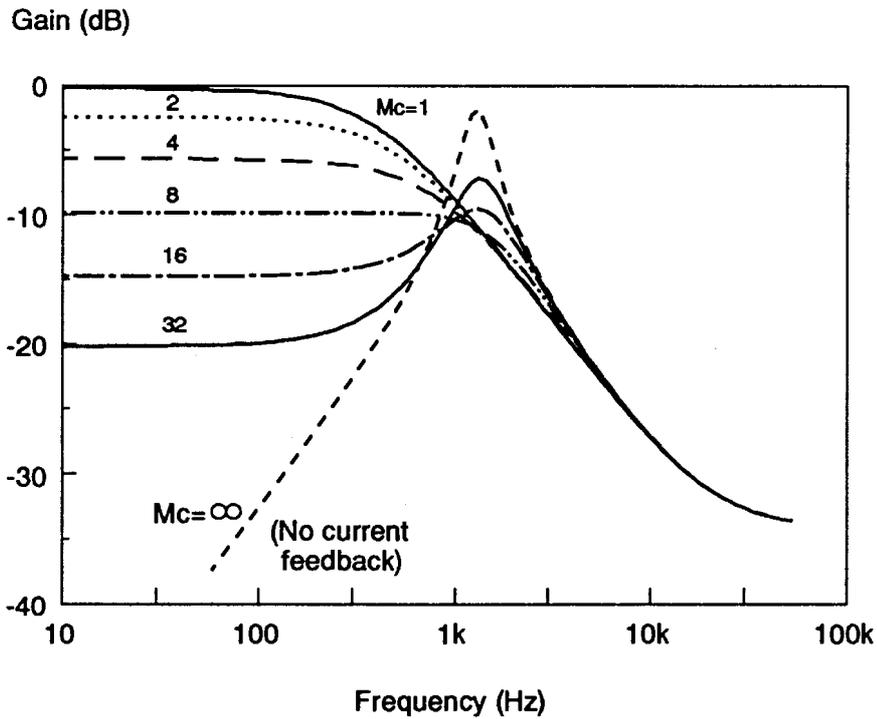
**Figure 5.17. Output Impedance of the Buck Converter:** Closing the current loop has the effect of increasing the output impedance of the converter below the resonant frequency of the filter. This is due to the tendency of the converter to maintain a fixed current when current-mode control is used. Adding an infinite external ramp reduces the current gain to zero, showing the voltage-mode characteristics of the power stage.
