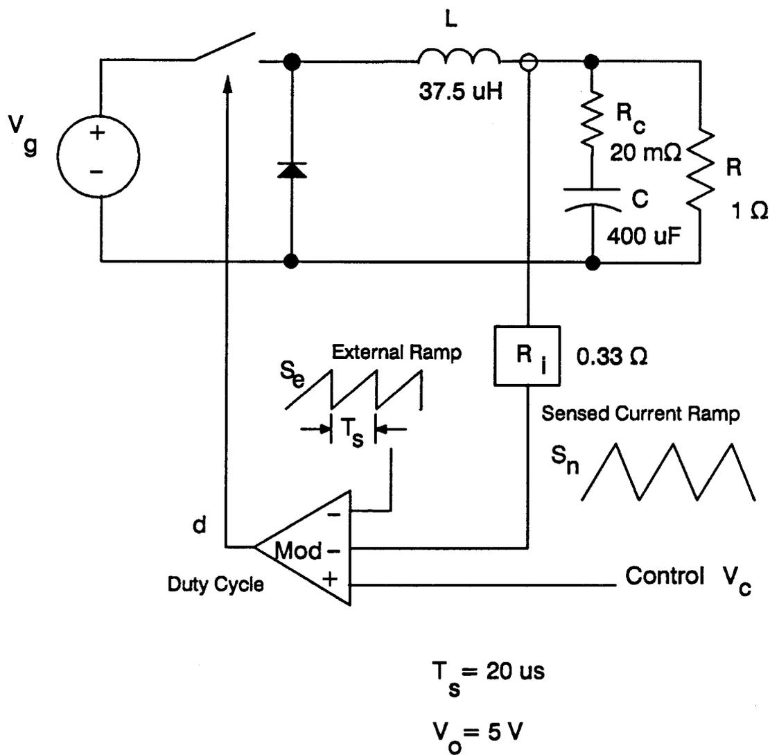
**Figure 5.1. Example Buck Converter for Confirmation of Small-Signal Predictions:** The buck converter has some of the most interesting characteristics with current-mode control and was chosen to confirm the modeling approach.
