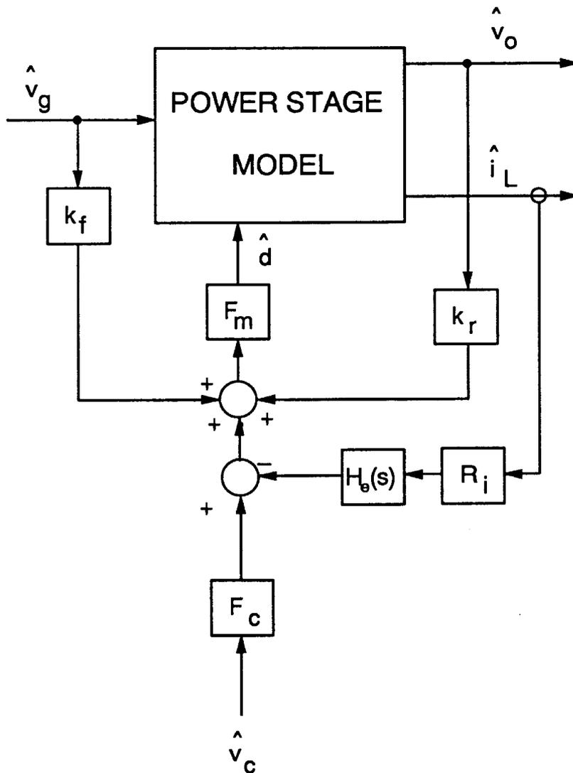
**Figure 4.5.** *Complete Small-Signal Model for Current-Mode Control:* Feedforward terms from the input and output voltages complete the small-signal model to predict the effect on inductor current of changes in the input and output voltage. This form of the model is useful for transfer-function analysis, and is used in Chapter 5.
