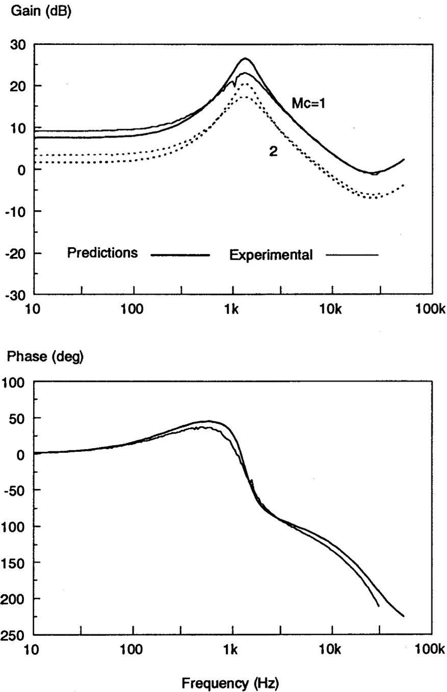
**Figure 5.5. Buck Converter Current Loop Gain - Experimental Results:** The predicted and experimental results for the current loop gain agree very well, especially at higher frequencies where average models fail to predict the current-loop instability.
