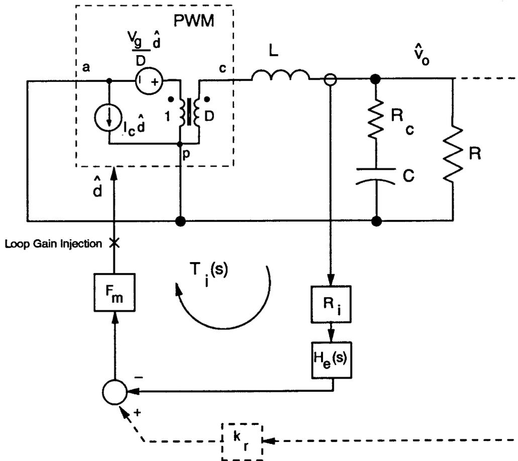
**Figure 5.3.** *Current Loop of the Buck Converter:* The feedback of the inductor current information creates a closed-loop system, the stability of which can be assessed by examining the current loop gain,  $T_i(s)$ . This loop gain is measured by breaking the feedback path at the output of the modulator gain,  $F_m$ .
