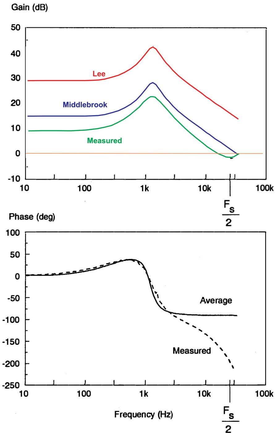
**Figure 2.16. Predictions of Current-Loop Gain Transfer Function:** Significant differences in measured results and predictions of two averaged models are shown here. Notice that both of the average models would indicate that the current-loop crossover frequency can exceed the Nyquist frequency of the system, yet still remain stable, a violation of basic Nyquist principles.
