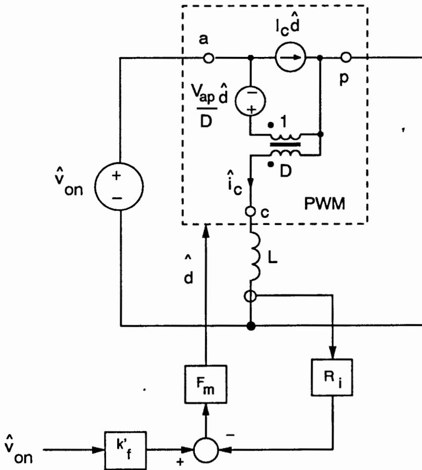
**Figure 4.8. Generic Current Cell with Fixed Voltage During Off-Time:** The on-time voltage, which is in general a linear combination of input and output voltages, is allowed to vary, and the value of feedforward term,  $k'_f$ , is derived for all converters.
