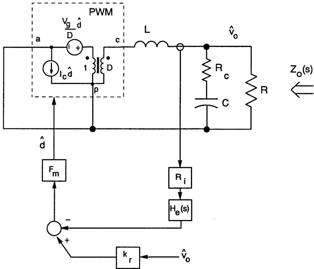
**Figure 5.16.** *Converter System with Current-Loop Closed and Load Current Perturbation:* The closed current loop will maintain the peak value of the current constant, and the output impedance is increased in the presence of current-mode control.
