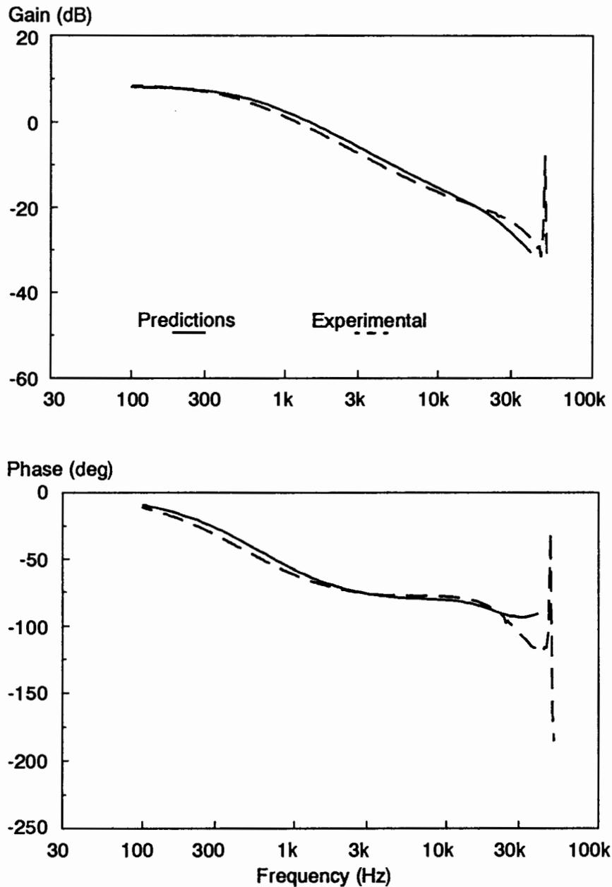
**Figure 5.22.** *Control-to-Output Measurement and Theory for Constant Off-Time,  $D=0.4$ : At higher duty cycles, the effect of the modulator phase lead  $F_c$  becomes significant. The double pole at half the switching frequency is still present in this transfer function.*
