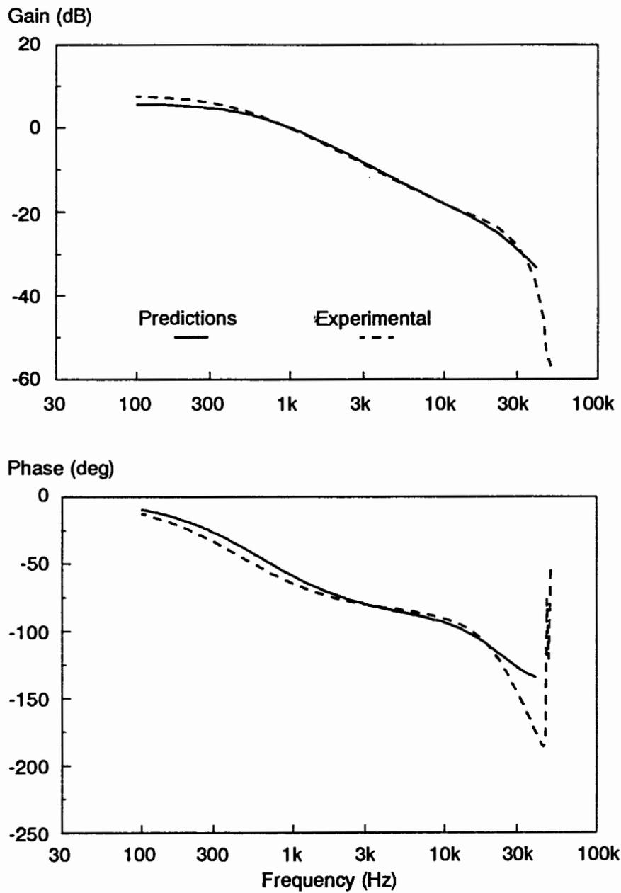
*Figure 5.21. Control-to-Output Measurement and Theory for Constant Off-Time,  $D=0.1$ : Measurement and theory agree very well for this transfer function up to 25 kHz, half the switching frequency.*
