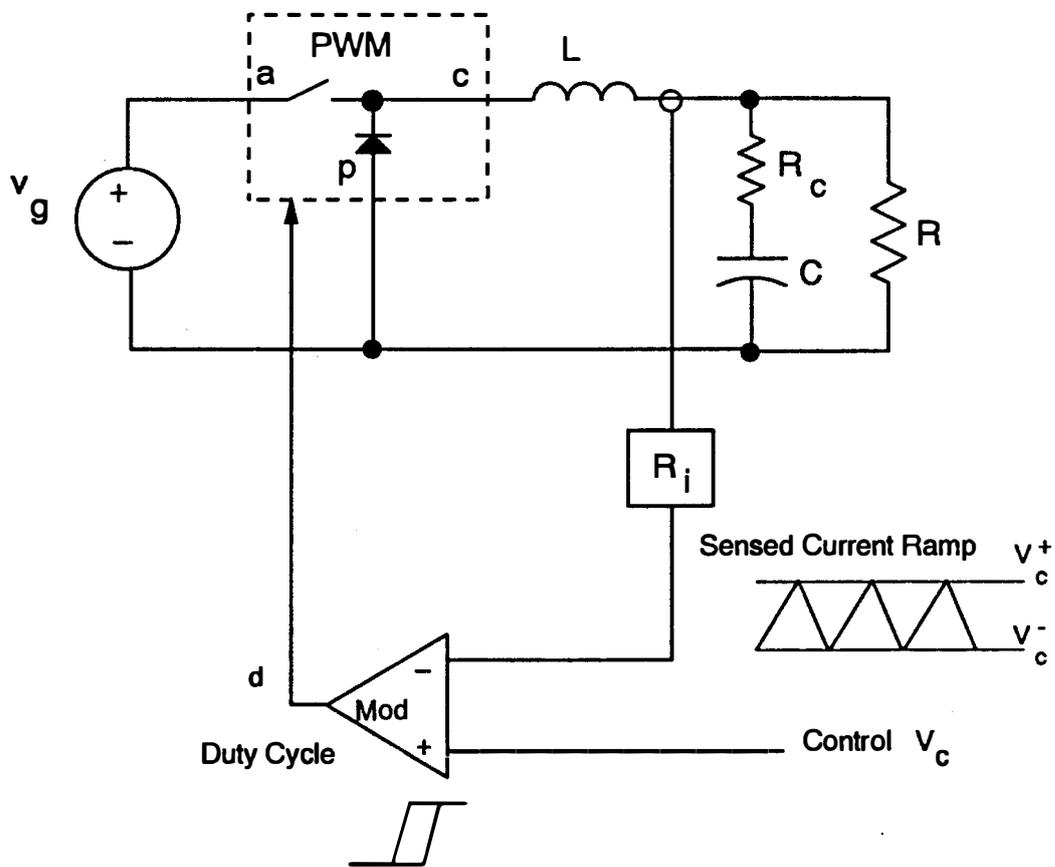
**Figure 2.2. Buck Converter with Hysteretic Current-Mode Control:** A control signal is used with a hysteresis band to determine the turn-on and turn-off times of the switch. No external clock or ramp is needed. This approach is not analyzed in this dissertation.
