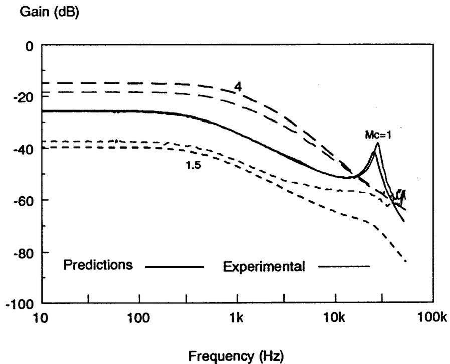
**Figure 5.15.** *Audiosusceptibility of the Buck Converter - Experimental Results:* Experimental measurements confirm the existence of the null value of the audiosusceptibility, although readings below the circuit noise level could not be attained. The measurements in the region of the null are very sensitive to any small changes in the slope of the external ramp.
