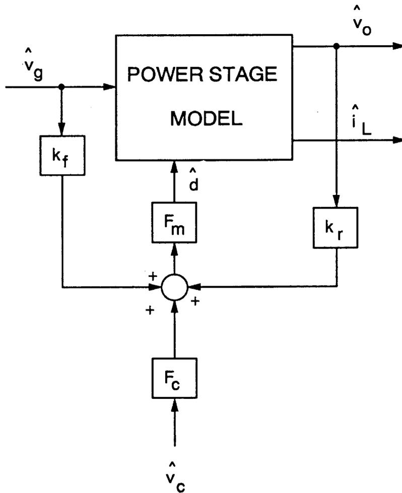
**Figure 4.12.** *Small-Signal Block Diagram for Current-Mode Control (DCM): There is no feedback of inductor current in this block diagram, and no sampled-data modeling is needed. The feedforward blocks,  $k_f$  and  $k_r$ , provide the necessary control information.*
