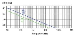
Figure 4b: Low Frequency Gain of Typical TL431 Circuit
