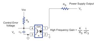
Figure 6a: TL431 High Frequency Gain Circuit
