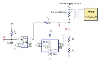
Figure 8: TL431 Loop Measurement Points
