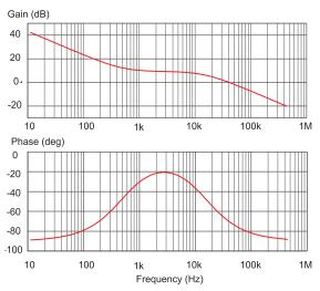
Figure 1b: Type II Compensation Bode Plot
