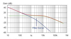
Figure 9b: Effect of Second-Stage Filter on Compensation Gain
