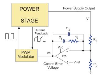
Figure 1a: Type II Compensation Feedback
