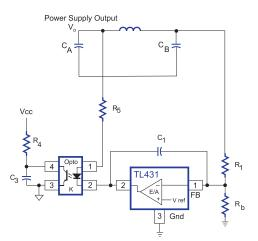
Figure 9a: Typical TL431 Configuration with Second-Stage Filter
