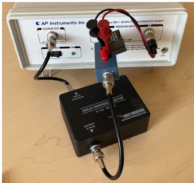
Figure 4: Measuring Inductor Rac Using AP300 Analyzer
