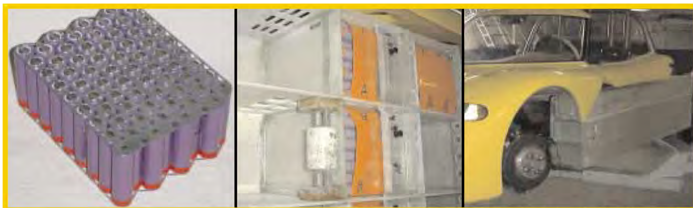
Fig. 9: AC Propulsion's Li-Ion battery pack components for the tzero. 6,800 cells are used in parallel-series combinations to provide the needed energy storage.
